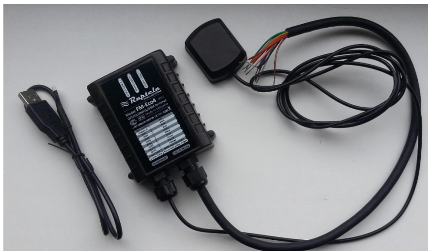
Figure 2. Box contents: ECO4/4+ device, GPS/GLONASS antenna, IO cable, USB cable (optional accessory)
