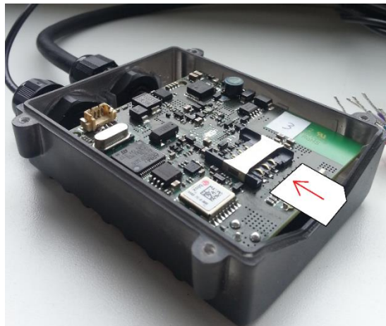
Figure 6. Insert SIM card into holder chip facing down
